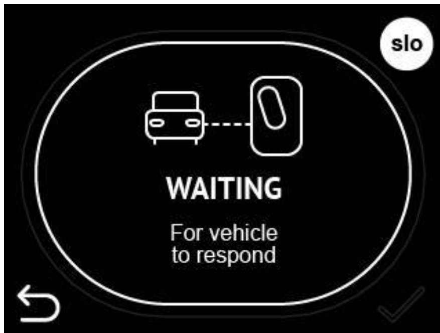
Figure 13: Charging station is waiting for EV to responds and starts charging
